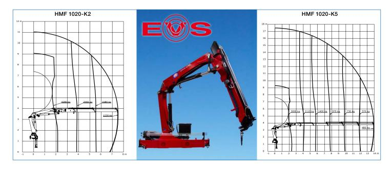
The HMF 1020-K with dual Power Plus link arm system, HDL-d speed adaptation system, RC-d proportional control valve with SC2 radio remote control for a very fast and precise handling. Fixed or variable flow pump.
