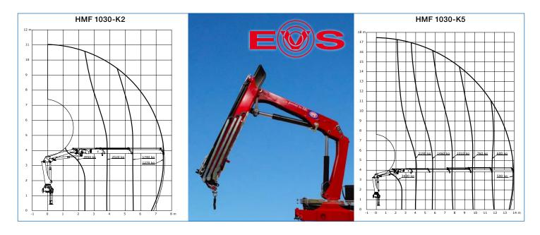
The HMF 1030-K with single Power Plus link arm system, HDL-d speed adaptation system, RC-d proportional control valve with SC2 radio remote control for a very fast and precise handling. Fixed or variable flow pump.
