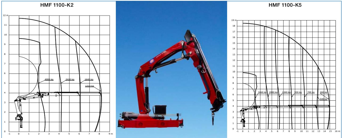
The HMF 1100-K model with dual Power Plus link arm system and manual ground control or stand-up controls and fixed flow pump.
