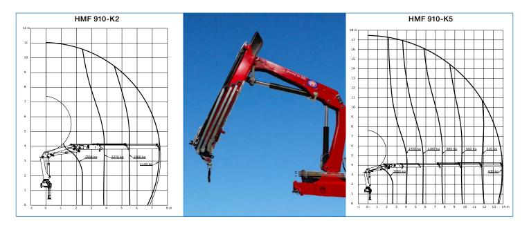
The HMF 910-K model with single Power Plus link arm system and manual ground control or stand-up controls and fixed flow pump.
