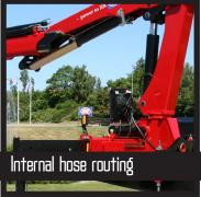
Hard wearing, nice and clean design with hydraulic hoses that are fed in nylon drag chains internally in the stabilizer beam. This offers a long life span as the hoses lie well protected against wear and squeezing damage.
